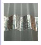
Polytape is a multipurpose repair tape used mostly for leaking roofs. It is a bitumen based self-adhesive tape with an aluminium foil finish to reflect the heat and light. It is smooth so it does not accumulate dirt. It can stick to almost any surface like concrete, metal, plastic, wood, glass e.t.c.
