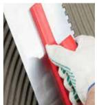
Polyflex parquet adhesive is a thick creamy based compound specially designed to bond parquet to concrete and wooden surfaces. it may also be used for bonding of tiles to floors.
